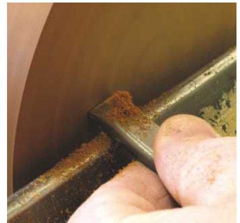
▲ Pic.6 The final finish on the top is done with a scrape with the skew chisel. This tool acts as a negative-rake scraper and on a dense timber like padauk will give a great finish
